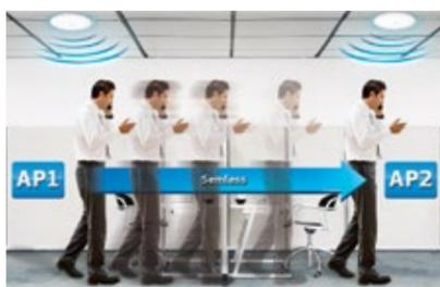
Samsung AirMove technology applies the handover methodology used within LTE mobile communications to deliver seamless roaming. Timing and choice of access point is determined centrally by the Access Point Controller (APC) which has a full picture of device activity and adjacent AP loading.
