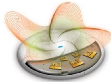
A Samsung 3 x 3 AP contains 15 antennas. Three antennas are used for RF monitoring and the remaining 12 provide an optimised RF pattern selecting a beam for each environment. As a result, dead areas are minimised, service coverage is expanded, and the receiving sensitivity is 2 dB higher than competitors' products. This means that the access point can accurately receive a signal from a mobile device with typically weak transmit power even when it is some distance away.
